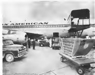
CONTAINERS are held up to 1,500 lb each and are lifted into the plane's forward cargo compartment by conventional lifting equipment. Trucks are floor lock containers into plane
